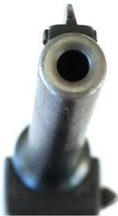
Another external indicator that this pistol has been modified is when viewing the barrel from the muzzle. The sleeve that has been placed in the barrel is very evident and clearly indicates that the barrel is no longer chambered for the 8mm round.
