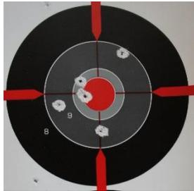
As for performance on the range, one has to remember that the Type-14 pistol was designed to be a combat arm and not a target pistol. With that in mind, I shot it a number of times and determined the point of aim at close range. I was able to shoot a couple decent groups with the target out at 10 yards by holding my point of aim approximately 6 inches below the center of the target.
