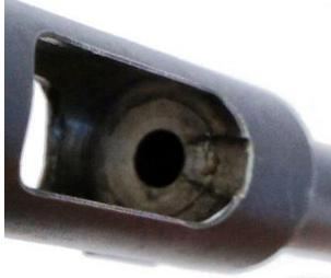
The sleeve that was inserted to make the conversion to the new caliber can be seen when viewing the chamber from inside the barrel housing.
