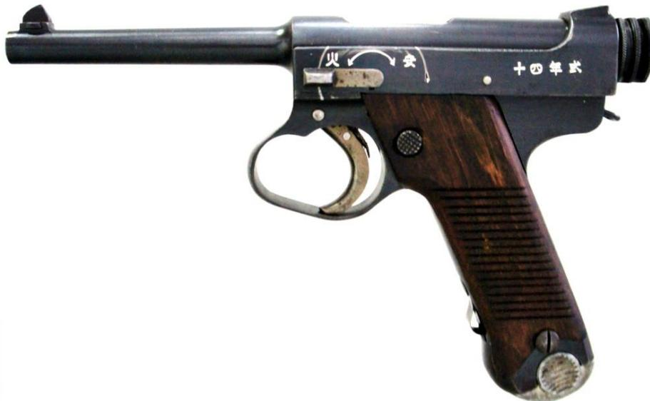
Almost simultaneously, with the change to the grip panels, a recess with corresponding cutout was machined into the front grip strap to accept an "S" shaped magazine retention spring. At the same time as the grip spring addition, a notch was cut into the
