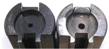
firing pin guides are also reported as serialized in this late production period. Any found loose 65mm firing pins with 0.08" tips and numbers on the barrel can be ascribed to late production.
