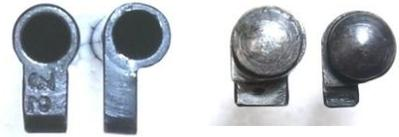
The next major firing pin design change occurred in July 1942 (17.7) when the firing pin was shortened from 73mm to 65mm for a longer striker fall. The firing pin guide length was correspondingly changed to a longer 54mm, and, the guide shape was also changed from flat sides to round sides (see
