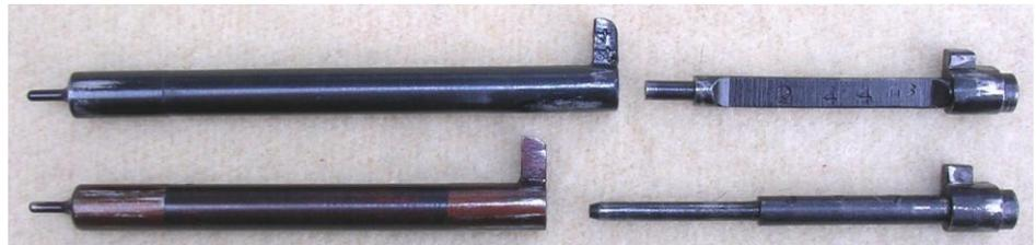
modifications, the firing pin guide did not change shape again with the round version lasting until the end of standard production. Both parts were number-matched to the individual pistol as before (pin numbered on the barrel; guide numbered on the side). Unnumbered firing pins and firing pin guides found in pistols during this period are replacements for the original parts. During March 1944 (19.3), the firing pin guide matching serialization was eliminated.
