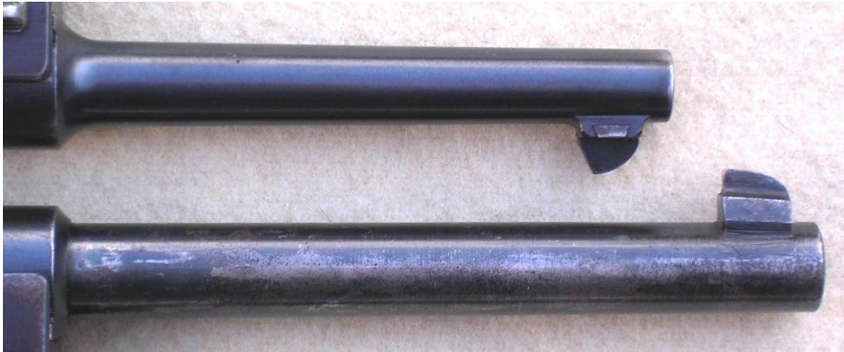
Some basic measurements show the difference in barrel sizes. The new tapered barrel is just less than one inch longer at 0.980" difference. The rear barrel diameters (measured 1/2" forward of the front slide boss) are 0.550" for the 8mm barrel and 0.625" for the new barrel. The front barrel diameters are 0.475" for the 8mm and 0.585" for the new barrel. From bore centerlines, the new barrel sight top is 0.030" higher.
